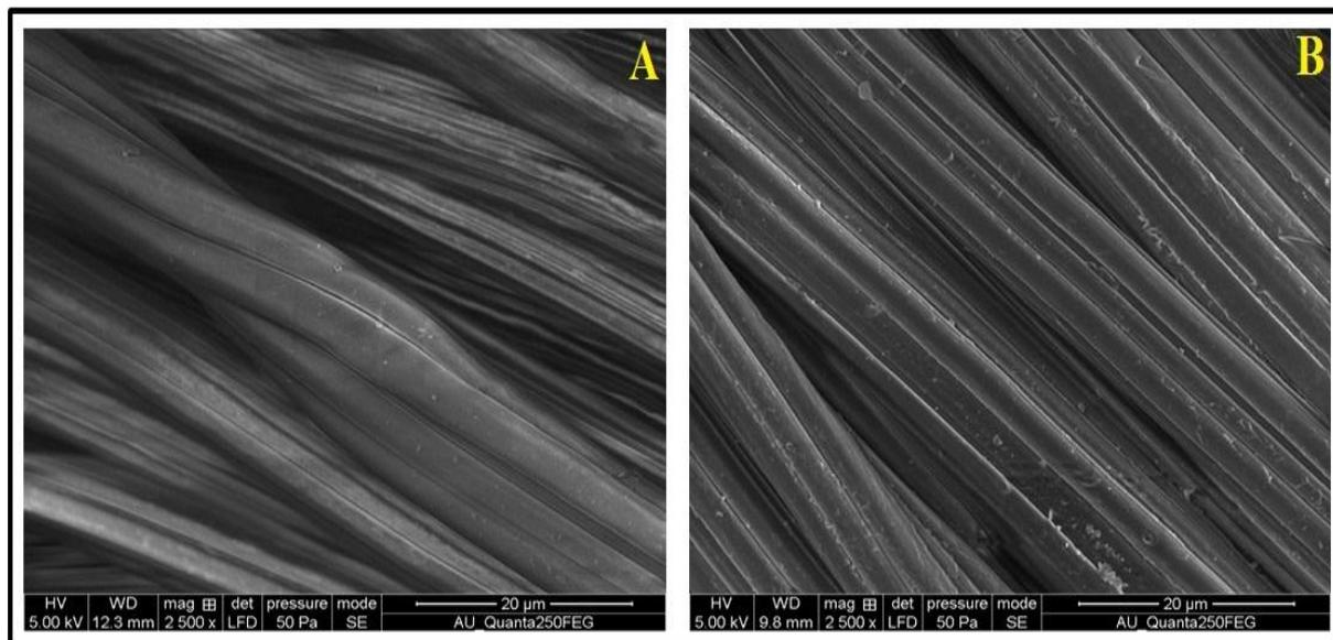
Fig. 3: HR SEM images A) Untreated bamboo fabric B) DC air plasma treated fabric
