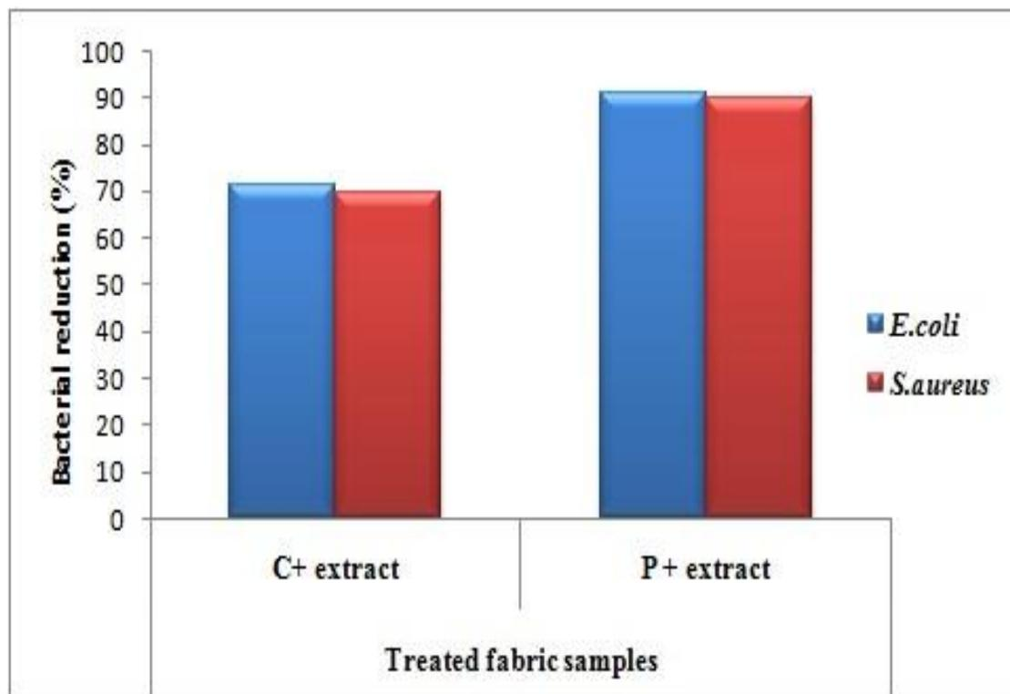
Fig. 5: Percentage reduction of the treated fabrics (AATCC 100)
