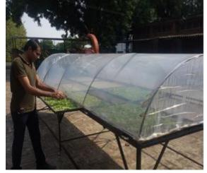
Fig. 2: Drying of mint leaves in solar tunnel dryer
