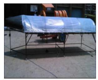
Fig. 1: Solar tunnel dryer
