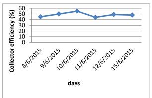
Fig. 5: Variations of solar Collector Efficiency
