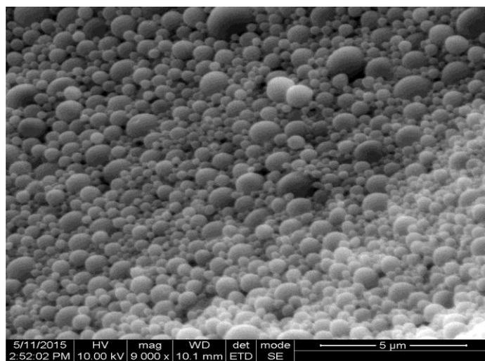
**Fig. 1: Morphology of PLGA nanoparticles visualized by scanning electron microscope - Magnification - 9000X**
