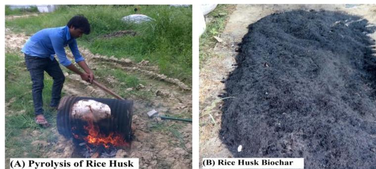
Fig. 1: Production of rice husk biochar by drum method as described by Srinivasarao *et al*.<sup>23</sup>
