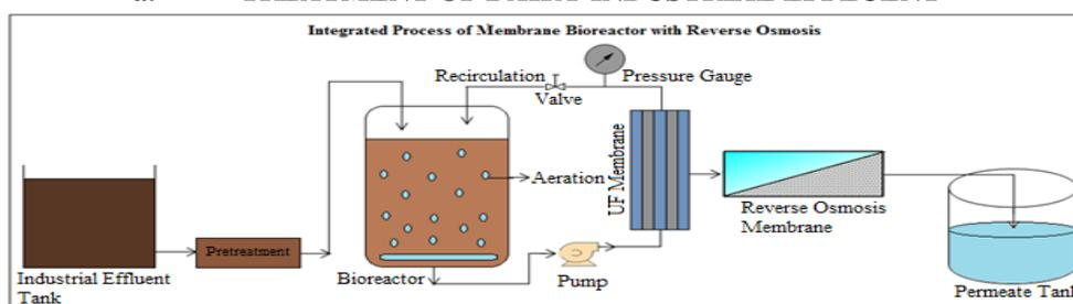
Fig. 1: Schematic diagram of aerobic integrated SSMBR+RO
