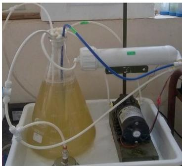
**Fig. 2: Experimental Setup of Side Stream Membrane Bioreactor (SSMBR)**
