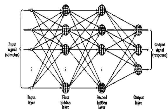
**Fig. 1: Architectural graph of multilayer perceptron**
