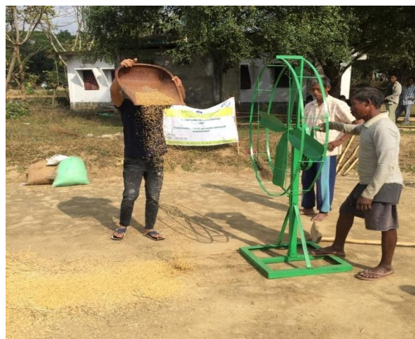
Fig. 4: Demonstration of hand operated winnower
