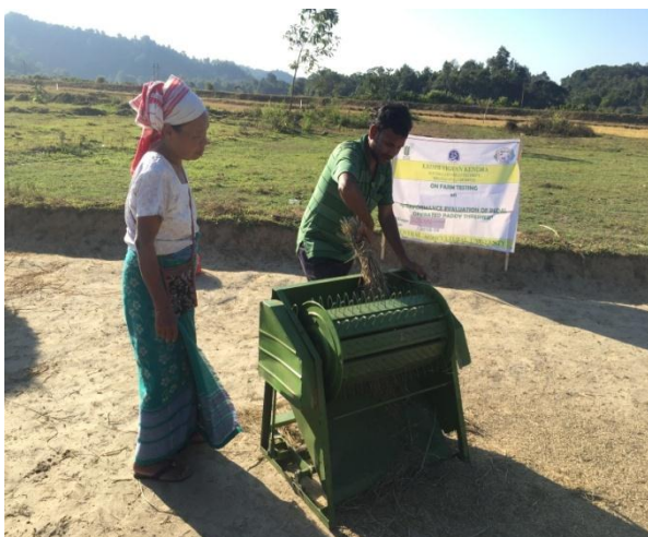
Fig. 3: Demonstration of pedal operated thresher Copyright © Sept.-Oct., 2020; IJPAB
