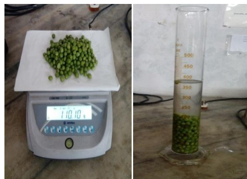
Fig 2.4 Measurement of True Density of Green Pea
