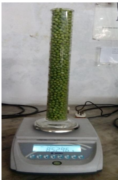
Fig 2.3 Measurement of Bulk Density of Green Pea
